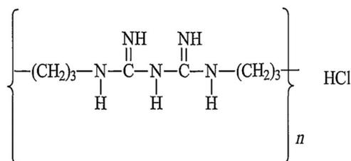
**Figure 3.** Chemical structure of PHMB.
